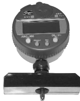
Special depth gage to measure dimple indentation on part surface. Gage's base modified to set correctly on part
